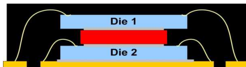
Fig. 6: stacked dice in a single package
