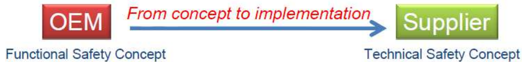
Fig. 3: the component supplier is normally responsible for ensuring the technical safety requirements for any given function [2]
