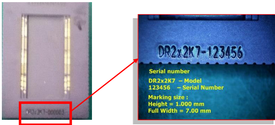
Fig.1 – Laser making example and serial number description
