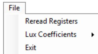
The **Reread Registers** function forces the program to re-read all of the control registers from the device and display them on the screen. This does not read the output data, because the program reads those registers continually while it is running.
