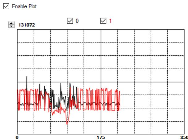
The scale of the Y-axis of the plot can be adjusted by clicking on the small up and down arrows at the top left corner of the plot. The scale can be set to any power of 2 from 64 through 65536.
