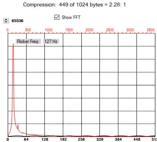
The scale of the Y-axis of the plot can be adjusted by clicking on the small up and down arrows at the top left corner of the plot. The scale can be set to any power of 2 from 16 to 16384.
