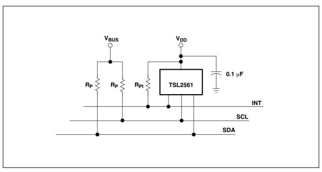
Pull-up resistors ( $R_p$ ) maintain the SDAH and SCLH lines at a *high* level when the bus is free and ensure the signals are pulled up from a low to a high level within the required rise time. For a complete description of I<sup>2</sup>C maximum and minimum  $R_p$  values, please review the I<sup>2</sup>C Specification at http://www.nxp.com.
