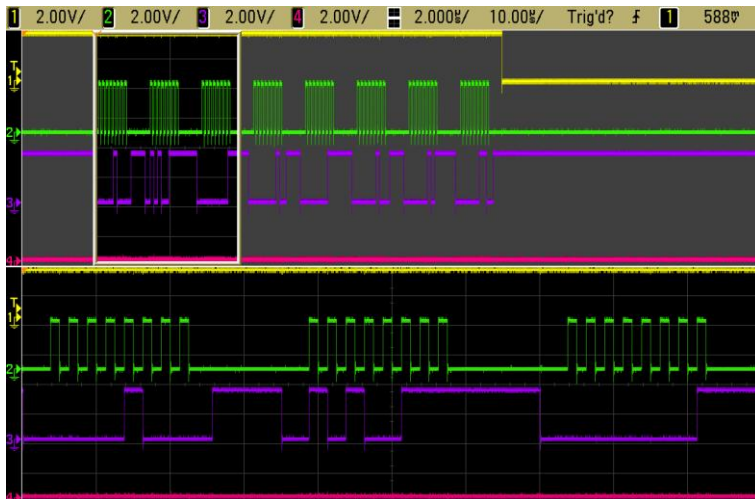
Figure 6: SPI Write Command - Page Mode
