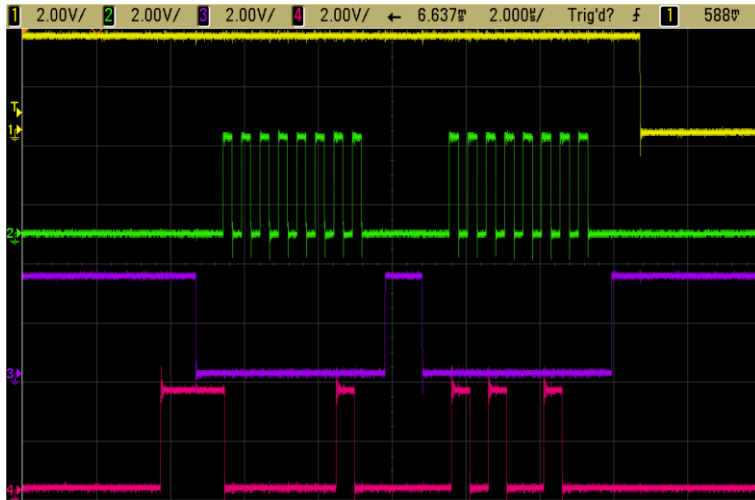
Figure 15: Direct Command Example: Get Temperature (Data read-out)
