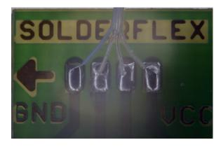
Figure 6 shows an example of the soldered wires on the 4-pin PCB connector, where the VSS/GND wire is on the most-left connector position and VCC is on its most-right.
