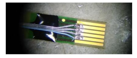
Figure 7 shows an example of the PCB Flex connector, where the colored VSS wire can be easily seen.
