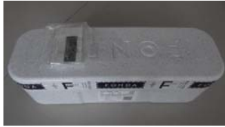
Fig. 4 RFID data logger (SL900A) on a box
