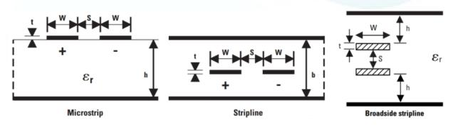
Use controlled impedance PCB traces that match the differential impedance of your transmission medium (e.g., cable) and termination resistor. Route the differential pair traces as close together as possible (use the minimum spacing "S" specified by your PCB vendor) and as soon as they leave the sensor. This helps to eliminate reflections and ensures that noise is coupled as common-mode.
