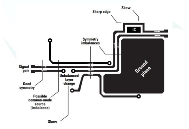
A conductor that carries current requires an opposite mirror current to return through some part of the system. This return current path will be the path of least resistance. For high-speed signals, the return current path will be the path of least inductance.
