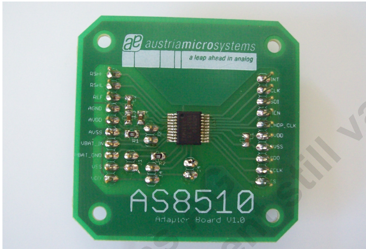
Picture 2: Adapter Board AS8510
