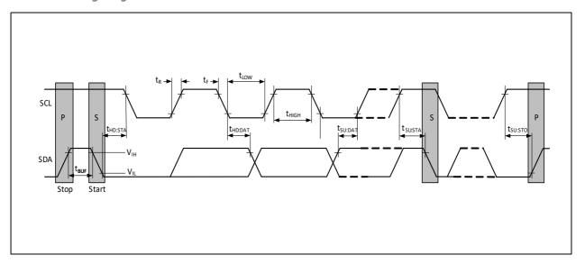
Figure 10: AS72651 SPI Timing Characteristics
