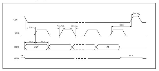
Figure 12: SPI Master Read Timing Diagram
