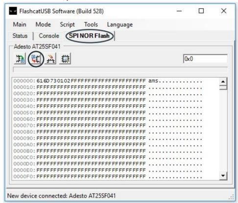
Then click the second button from left for programming the device. The file selection window will show up and please select the firmware you would like to program into the device and click 'OK". With the flashCat choose always the complete .bin file. Then click "OK" on the small window, which allows you to set Base Address and Length. We would take the default value as shown in the window below.
