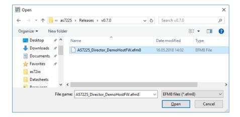
After clicking on the "Open" button, the selected file is shown in the "Host Controller Firmware" box. Now, click on the "Run FW Update" button to start the firmware update. The software calls a background console tool for the firmware upload. It is finished after a few seconds.
