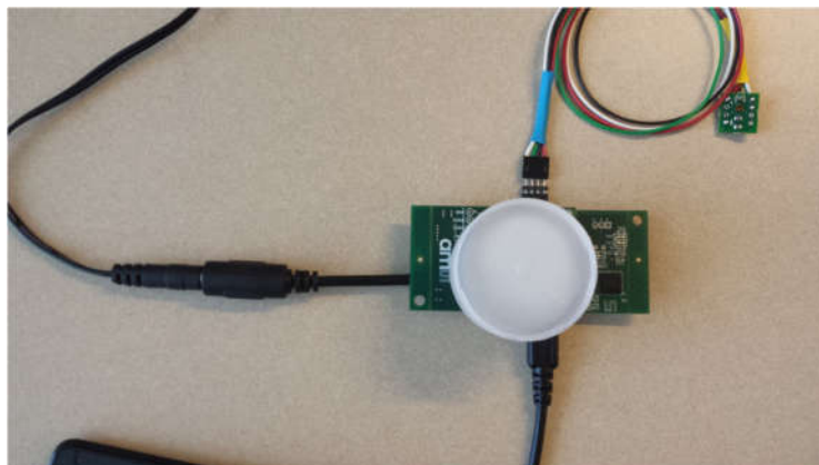
Figure 2. AS7221 SLIK & AS4531 – Connected to PC & DC Power
