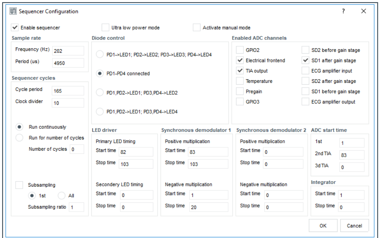
Figure 3: Sequencer Configuration for NTC Temperature Sensor
