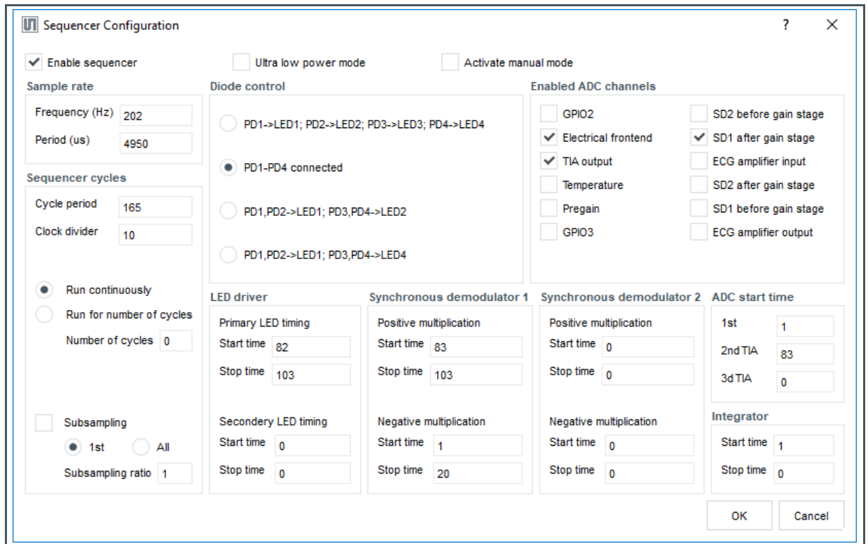
Figure 2: Sequencer Configuration for NTC Temperature Sensor
