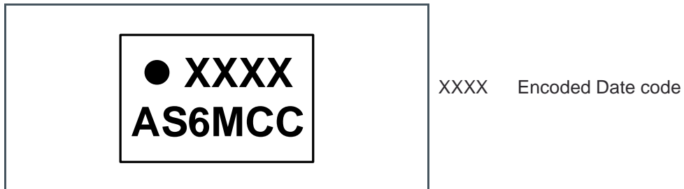
Figure 37: WLCSP Package Marking/Code
