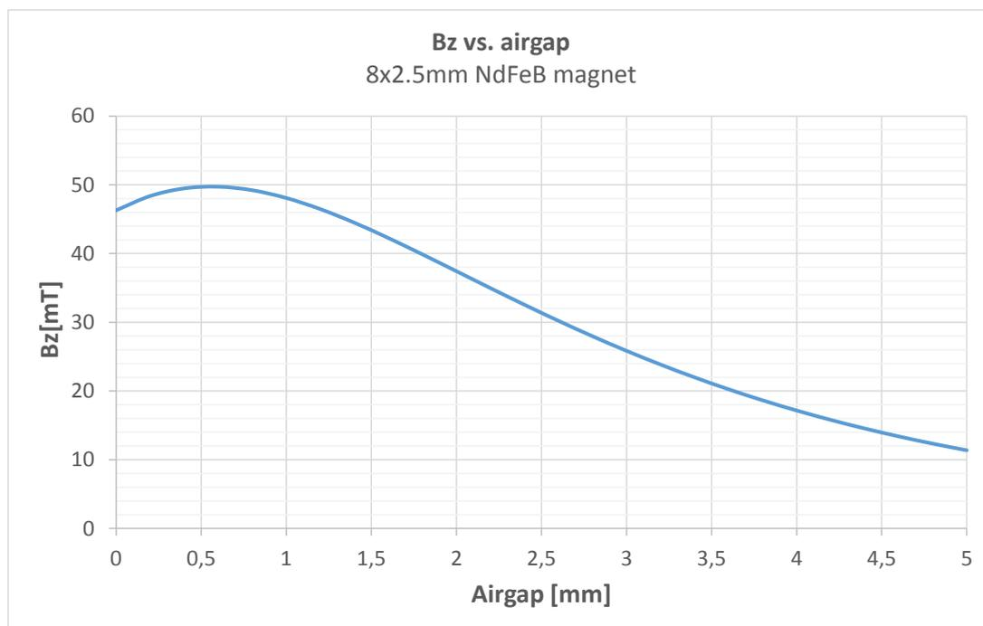
Figure 3: Magnetic simulation of magnetic field Bz versus the mechanical airgap
