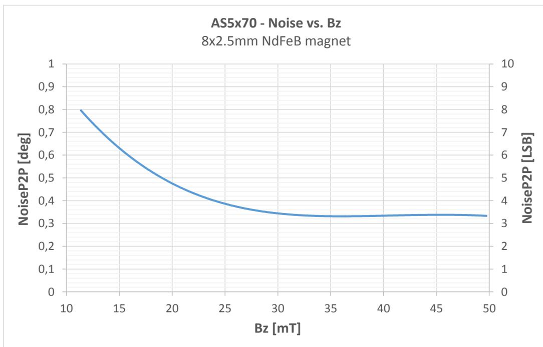
Figure 4: Noise performance versus magnetic field  $B_z$
