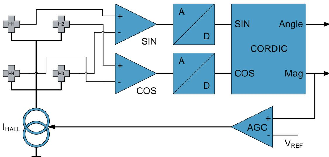
Figure 2: Signal path block diagram of AMS magnetic position sensors
