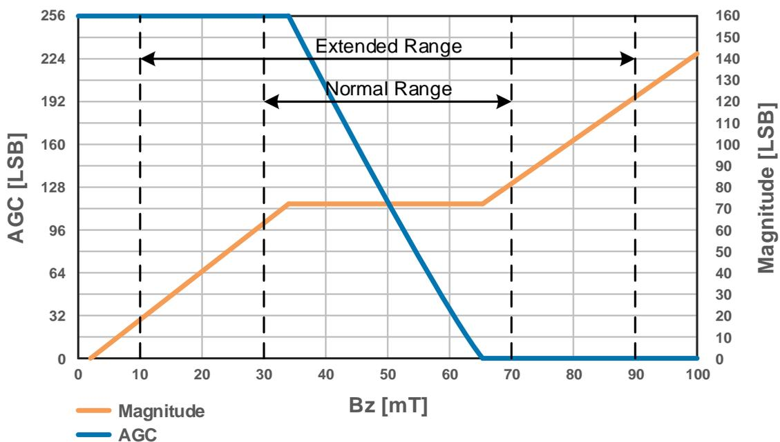
Figure 1: Typical relationship between AGC, Magnitude and magnetic field strength
