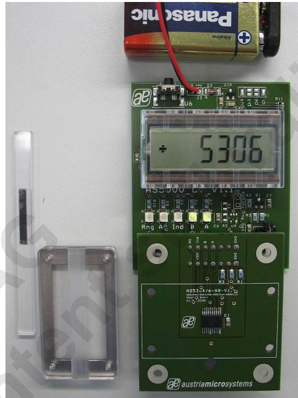
Fig. 2: AS5306 Evaluation Kit with 1.2mm pole length magnet
