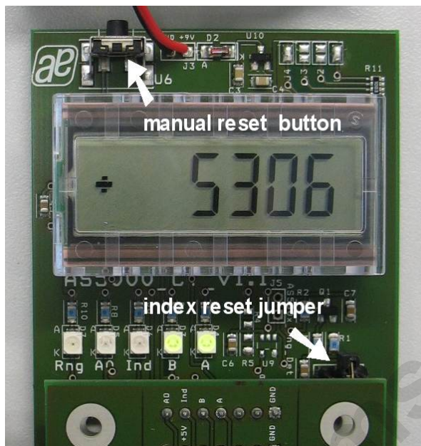
Fig. 3 : the counter module with reset button and jumper
