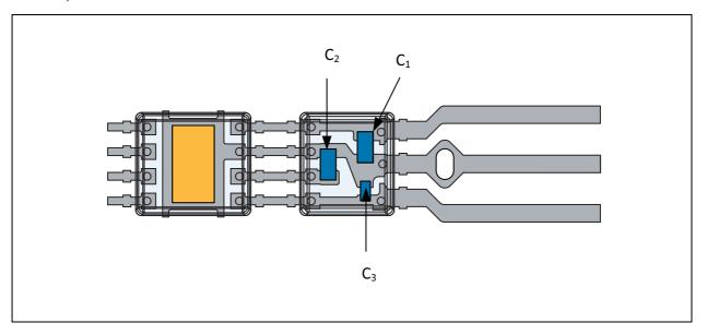
The built-in capacitors are ceramic multilayer type X8R. The capacitors build for high temperature applications up to 150°C
