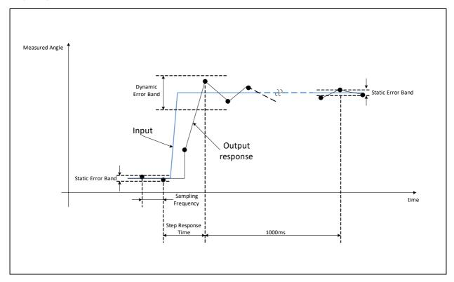
It is possible to optimize the step response time versus the dynamic error band with the FILTER setting.
