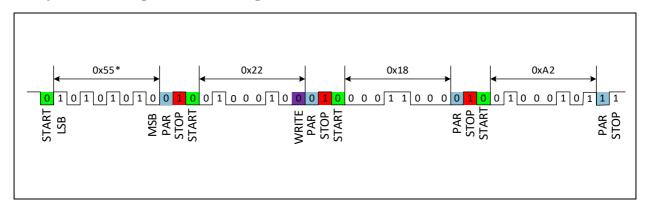
Figure 22: Example of Read (Reg[0x2B], Reg[0x2C])
