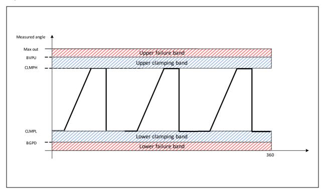
Figure 31: Quadruple Quadrant Mode
