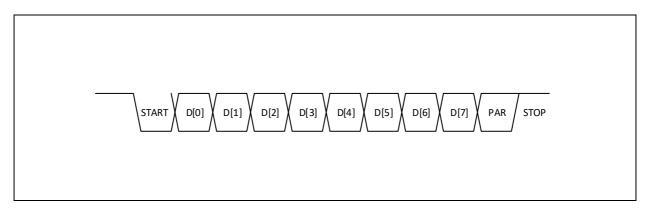
The PAR bit is even parity calculated over the data bits (D[0:7]). Each frame is transferred from LSB to MSB.
