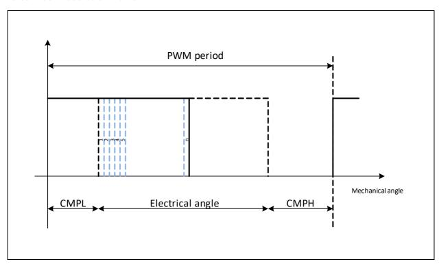
The PWMFR setting sets the duration of the PWM frequency. The PWMSR setting chooses between fast and slow steps.
