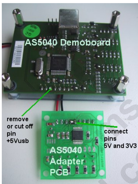
Figure 9: configuring the Adapter PCB for 3.3V operation
