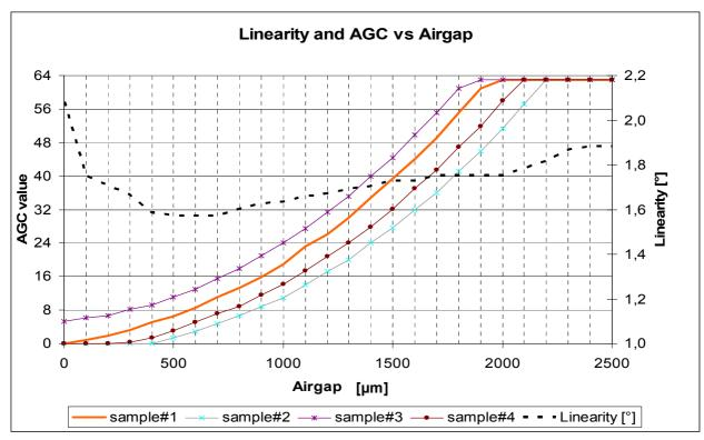
As shown in Figure 59, the AGC value (left Y-axis) increases with vertical distance of the magnet.
