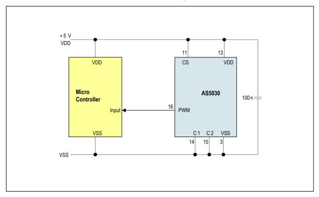
The minimum PWM pulse width  $t_{ON}$  (PWM = high) is 1 LSB @ 0° (Angle reading =  $00_H$ ).
