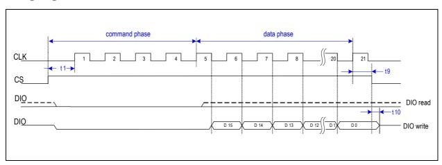
Figure 25: Serial Bit Sequence (16-bit read/write)
