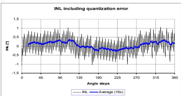
Figure 58 shows a typical example of an error curve over a full turn of 360° at a given X-Y displacement. The curve includes the quantization error, transition noise and the system error. The total error is  $\sim 2.2^{\circ}$  peak/peak ( $\pm$  1.1°).
