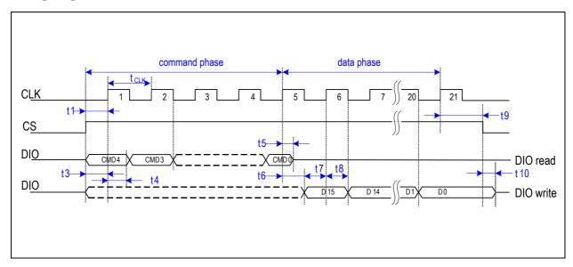
Figure 22: Serial Bit Sequence (16-bit read/write)
