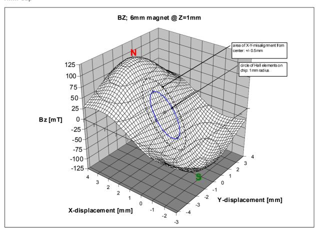
Figure 62 shows the same vertical field component as Figure 61, but in a 3-dimensional view over an area of  $\pm$  4mm from the rotational axis.
