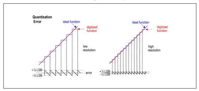
The resolution of the encoder determines the smallest step size. The angle error caused by quantization cannot get better than  $\pm \frac{1}{2}$  LSB. As shown in Figure 57, a higher resolution system (right picture) has a smaller quantization error, as the step size is smaller.
