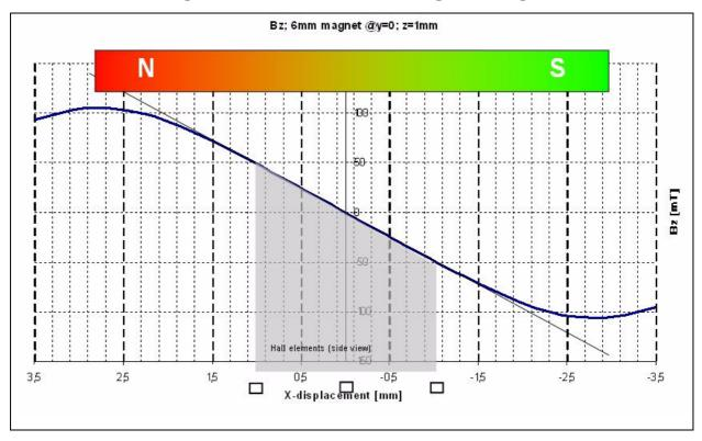
Figure 61 shows a cross sectional view of the vertical magnetic field component Bz between the north and south pole of a 6mm diameter magnet, measured at a vertical distance of 1mm. The poles of the magnet (maximum level) are about 2.8mm from the magnet center, which is almost at the outer magnet edges. The magnetic field reaches a peak amplitude of  $\sim \pm 106$ mT at the poles.
