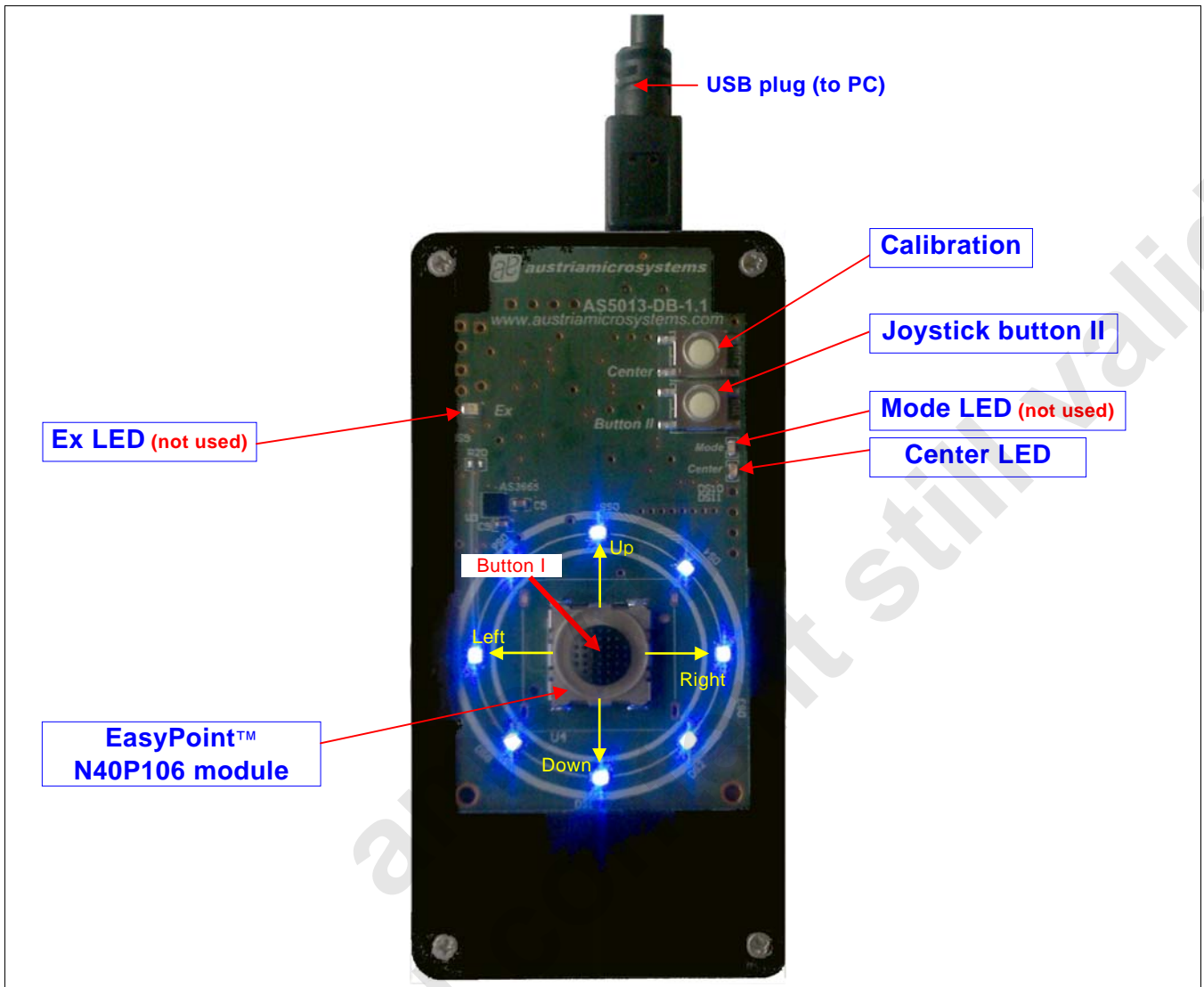
Figure 2. AS5013 Demoboard, technical description
