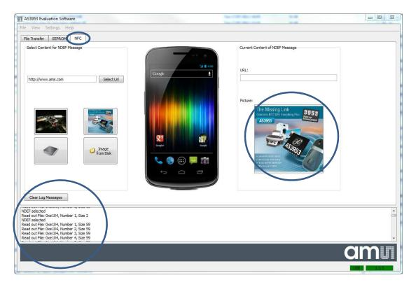
File/URL Transfer from GUI to Phone: open the amsNFC app and click on "transfer image" or "transfer Url". Select an image or url respectively and place the phone on the AS3953 GP demo antenna. The file transfer starts automatically.
