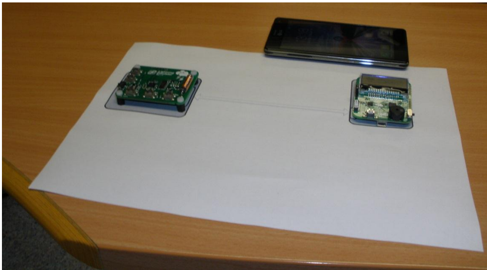
Figure 7: The cell phone is too close to the Lightning Sensor Board. Especially when the cell phone's display is turned on the Lightning Sensor Board will not work as intended.
