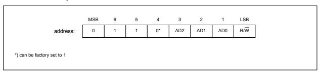
The bit 1, 2 and 3 of the address byte are defined through the resistor @ the device select pin ADDR (see Figure 30). A maximum of 8 devices with the same pre-set code can be connected on the same bus at one time.
