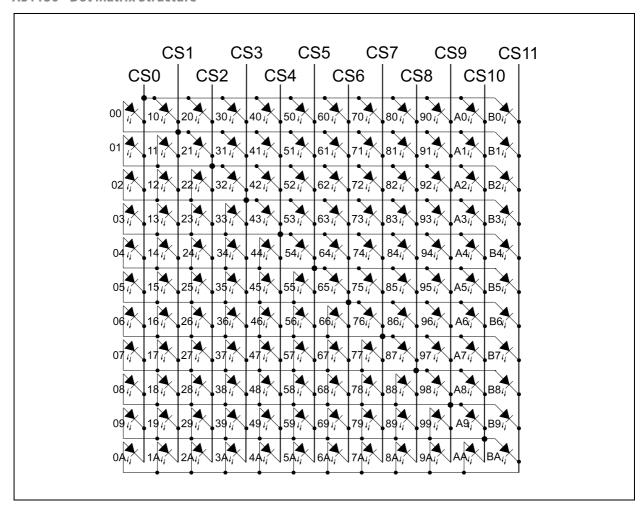
In Figure 34 it is described which databit represents which LED in the matrix. Per default all databits are '0', meaning no LED is on. A '1' puts the LED on.
