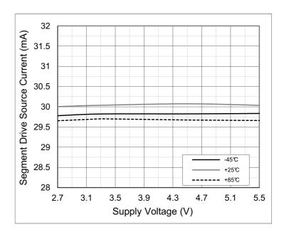
Figure 12: Segment Drive Current vs. Temperature
