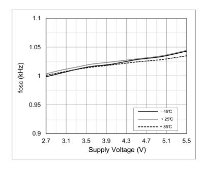
Figure 22: Oscillator Frequency vs. Temperature
