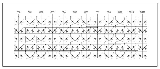
In the movie display mode the frame is shown in the matrix at once. On the contrary in the scroll function the frame is shifted through the matrix segment after segment (CS0 to CS1 to CS2 to CS3...).
